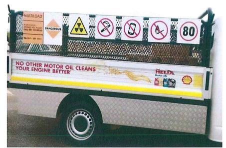
The vehicle on the previous page is transporting engine oil (flammable liquids). List 4 (four) things that are INCORRECT about the placarding. (4)
