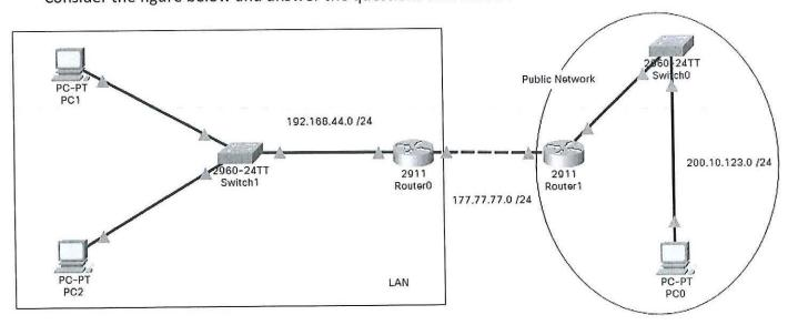
10.1 Configure a static default route on both routers so that the routers can direct traffic to their destinations respectively. [4]
